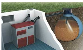
Silo enterré (source Biotech)
